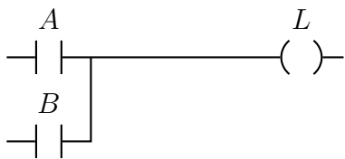
Figure 12: A simple ladder logic example (Hugh jack at English Wiki-books, file Trial_ladder_logic.svg ).
